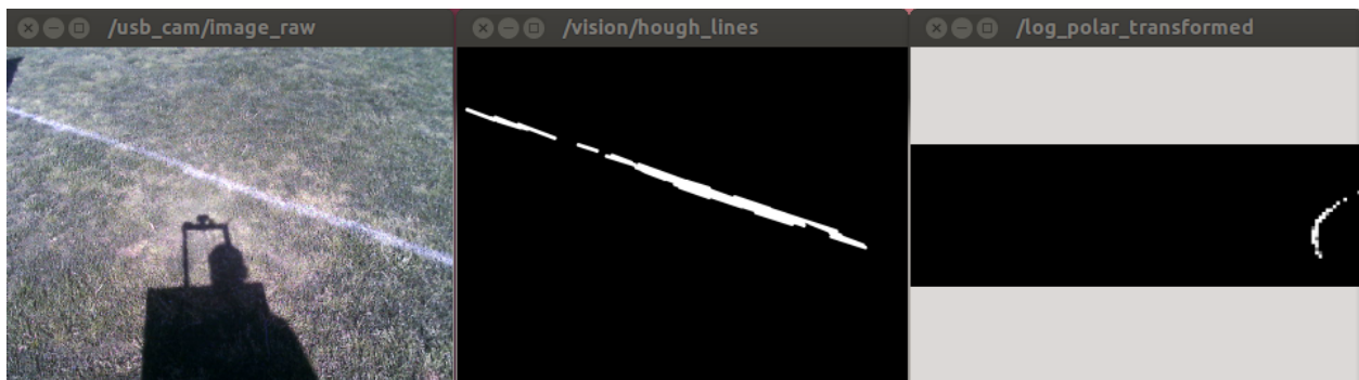
Figure 3: middle: detecting lanes using hough lines, right: log-polar transform on binary image
